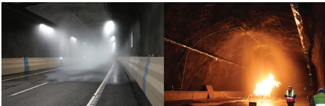
The T-REX (TN) system consists of a single ceiling water pipe attached to horizontal nozzles every five metres which spray large droplets in a sideways direction, covering the entire tunnel cross section.
