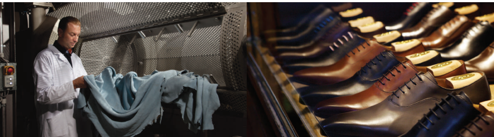
CLEANTAN process makes it possible to tan leather with compressed CO 2 without having waste water and is easy to integrate in running tanneries.
