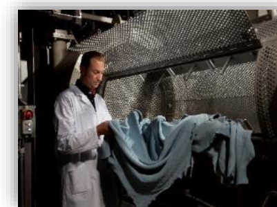
Tan leather without waste water by using CO 2
